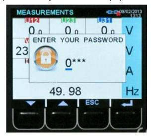
A 4 digit password must be entered using buttons. The factory default password is "9876". The buttons modify the value of the current digit. The button steps to the next digit.
