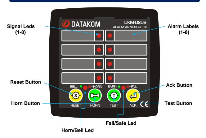
SIGNAL LEDs: There are 8 red/green adjustable signal leds on the panel. According to the input signal and pressed pushbutton,leds can be on Fast Flash, Slow Flash, Steady On and Off states.
