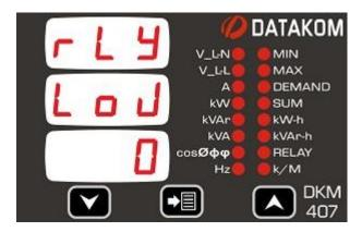
The relay output is the combination of 4 functions defined above. Thus various combined functions may be attributed to the relay output.
