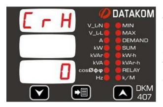
This parameter sets the high limit for overcurrent alarm.
