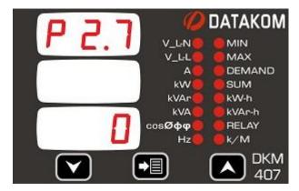
The device firmware version is displayed as shown in the lefthand figure.
