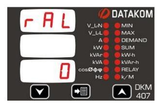
This parameter sets the low limit for low reactive power alarm.
