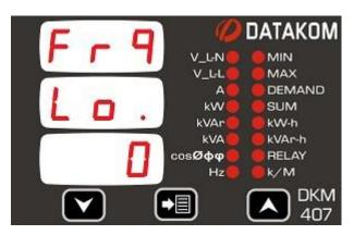
This parameter sets the low limit for low frequency alarm.
