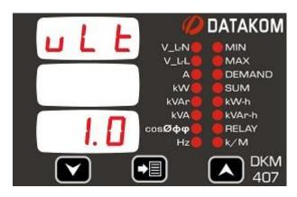
This parameter sets the ratio of voltage transformers.
