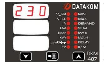
The calibration screen for L1 phase voltage will appear. 1 second after, the coefficient used for measuring the voltage will appear in displays 2 and 3.
