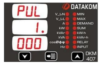
This parameter determines the amount of kWh (or kVArh) for 1 pulse output.
