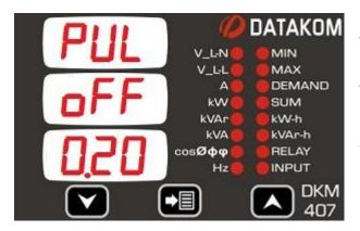
This parameter determines the minimum rest duration between two pulses.
