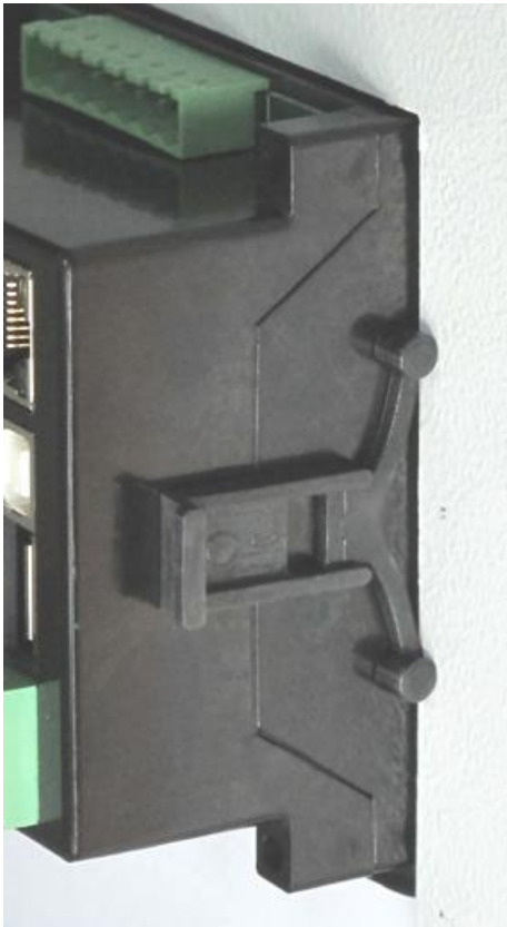
Installation of self retaining type bracket
