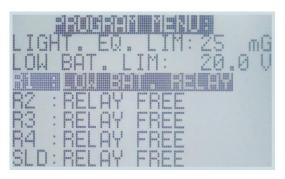
Modified parameters are saved to a non-volatile memory and are not affected by energy failures.
